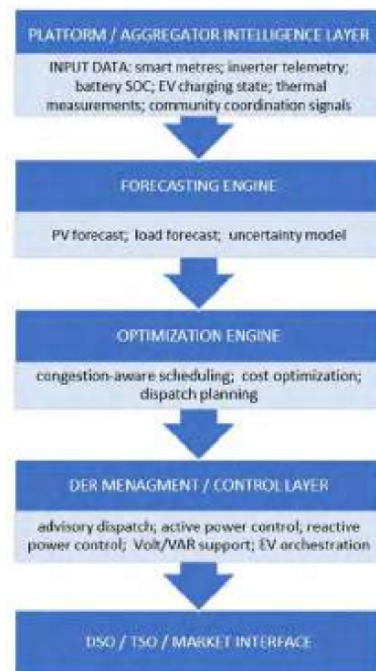
Figure 3.3 Platform / Aggregator Intelligence Layer
