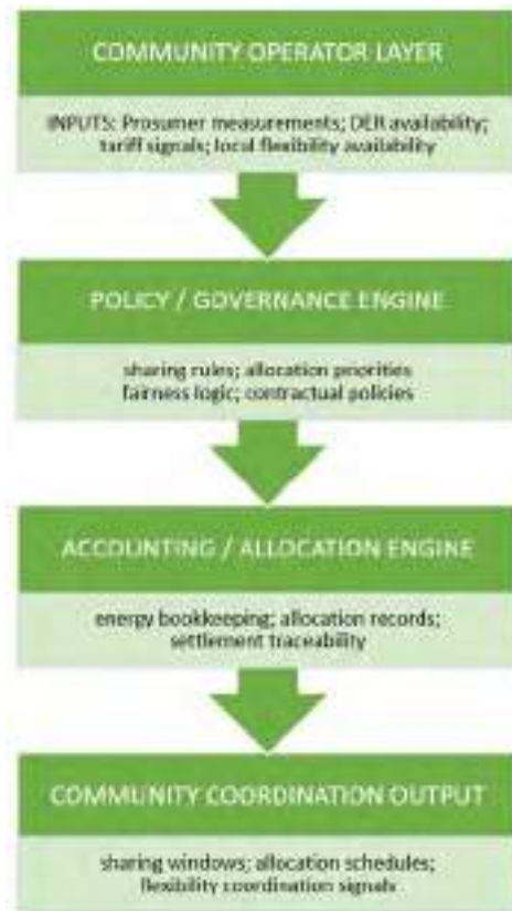
Figure 3.2 Community Operator Layer: Sharing Logic, Allocation, and Accounting
